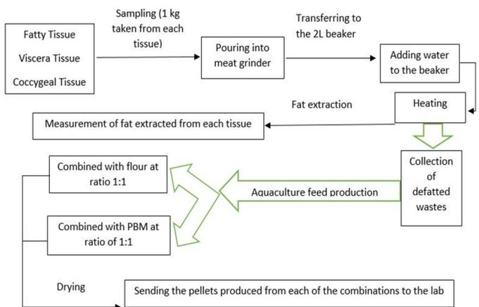
Figure 1. Overview of poultry waste processing operations.
